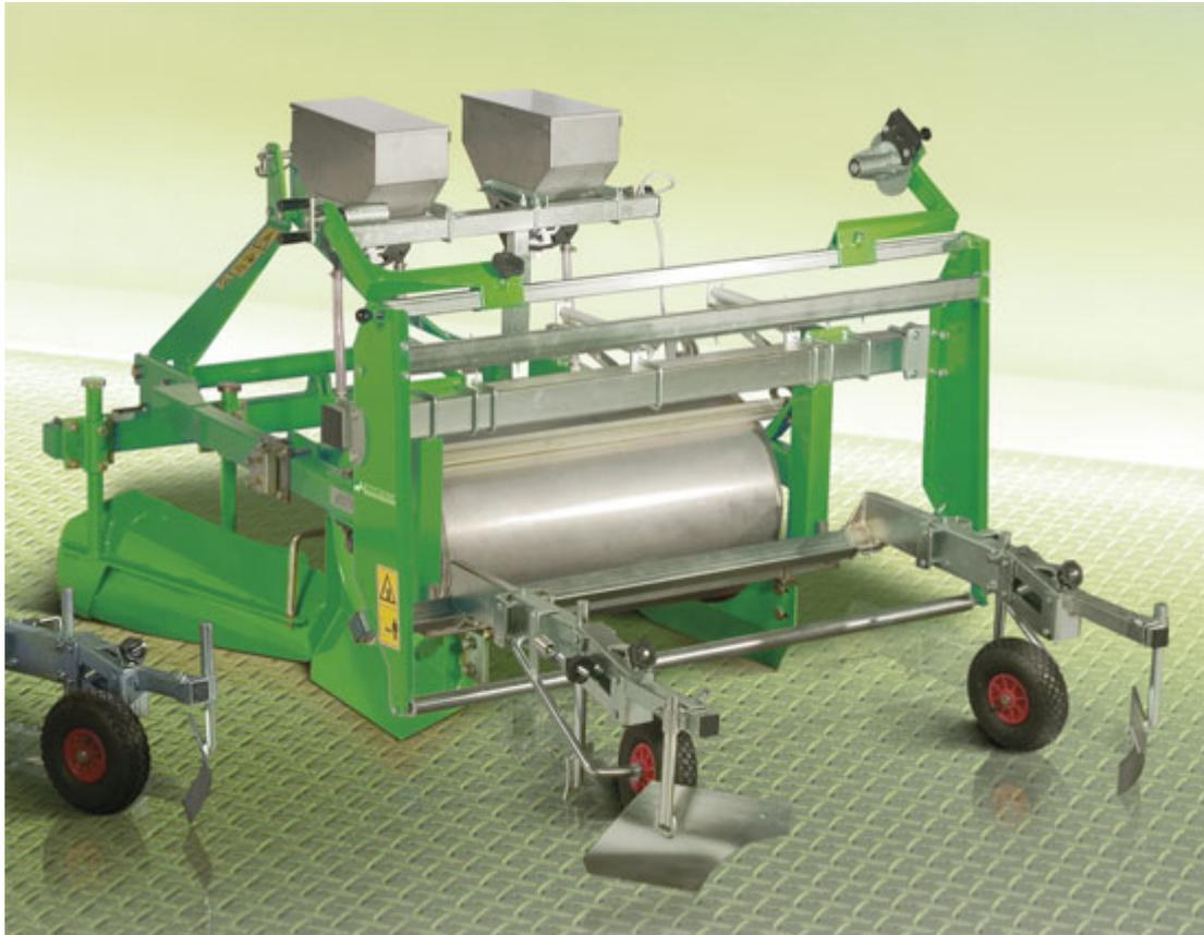
The bed former AB shapes the bed through a system with shares and presses the soil with a roller. The strong frame makes the machine suitable to work on any kind of soil. AB is fast and easily adjustable in height and width. The bed former mulch system layer AP can work any kind of soil. It forms the bed through a system made up of a share system and a sturdy roller presses the soil.
